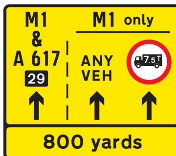
Lane restrictions at road works ahead
