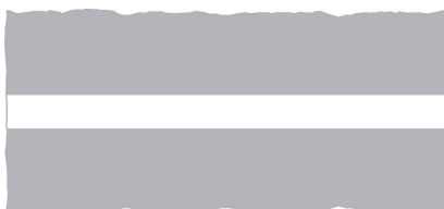
Stop line at 'Stop' sign
