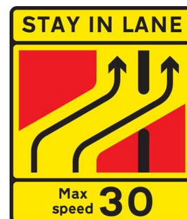
One lane crossover at contraflow road works
